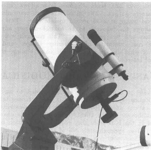
Figure 1. The remotely-controlled 16-inch telescope of the Sommers-Bausch Observatory of the University of Colorado at Boulder.
