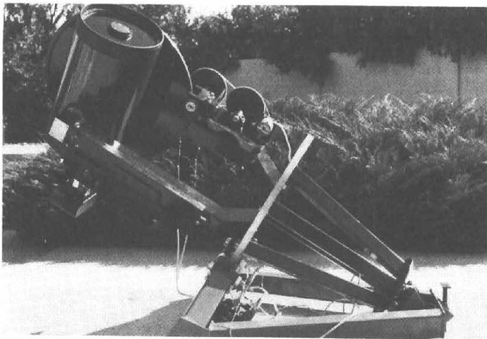
Figure 2. AutoScope mount for 0.5-meter telescopes. Shown with 0.25-meter optics—one of three with these smaller optics built for the Jet Propulsion Laboratory. The mount employs 24-inch diameter friction driven disks in both RA and Dec for the final drive, and two stages of precision Berg-belt reduction. This allows very smooth, totally backlash free operation without preloading—ideal for computerized control.
