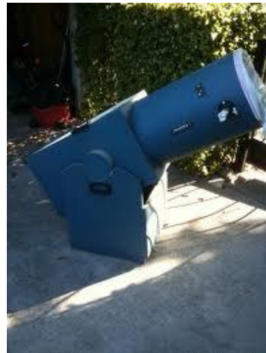
Star testing and mirror mount test stand. An original Coulter 13. My F3 mirror is a slumped Coulter mirror.
